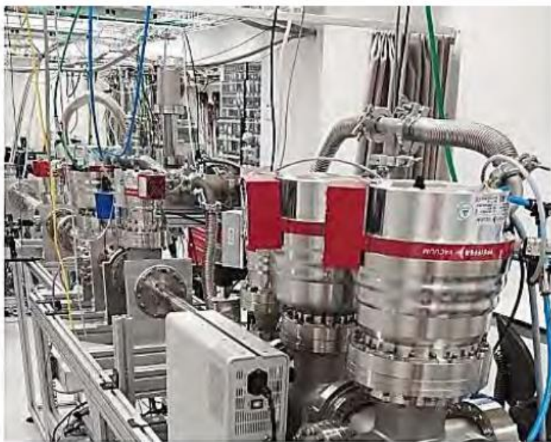
The four-and-a-half-meter-long experimental setup starting with the supersonic beam of...
